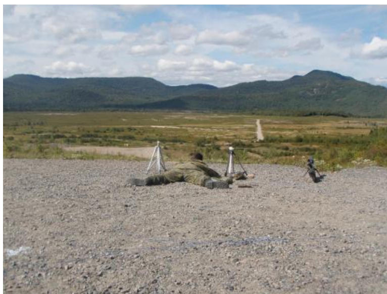
Figure 3: Measurement positions of the C8, C14, C15 and C16 weapon noise at CFB Valcartier (top), and photo of the range environment (bottom). Microphones were placed close to the shooter and on tripods at 4 m increments. The gravel-covered ground surface is partially sound-absorbent, and there are no reflective surfaces near the weapon.
