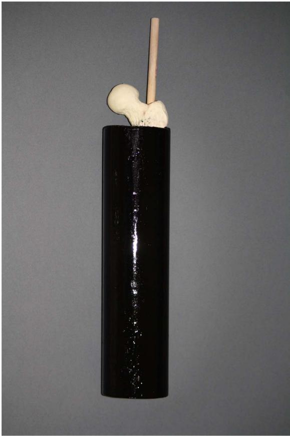
**Figure 2** Composite femur encased in black gelatine matrix, completely obscuring underlying fractures.
