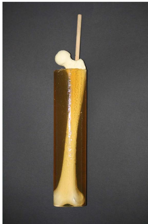
**Figure 1** Composite femur encased in clear gelatine matrix. Wood dowels were inserted and epoxied into the piriformis fossa to facilitate handling of the specimens.
